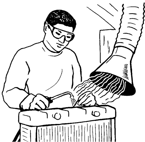
Local Exhaust Ventilation
